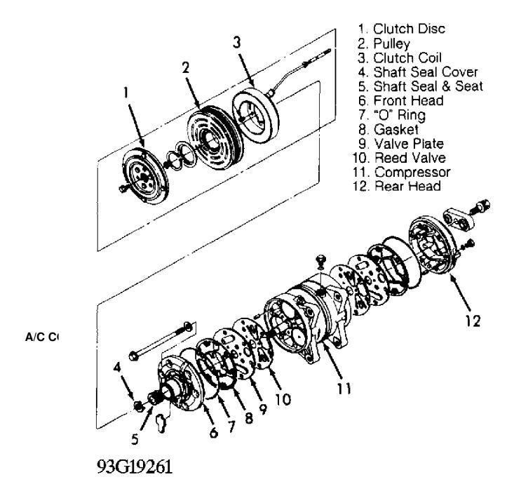
Fig. 5: Exploded View Of Compressor (Diesel Kiki 6-Cylinder) Courtesy of Isuzu Motor Co.
