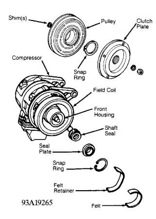
Fig. 13: Exploded View Of Typical Compressor (Nippondenso 10-Cyl) Courtesy of Ford Motor Co.
