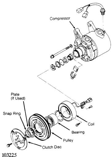
Fig. 4: Exploded View Of Rotary Vane Compressor (Diesel Kiki) Courtesy of Nissan Motor Co., U.S.A.
