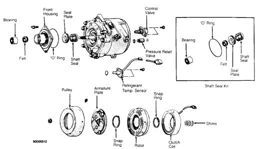
Fig. 17: View Of Compressor (Sanden Scroll-Chrysler & Mitsubishi Shown; Honda & Hyundai Similar)
