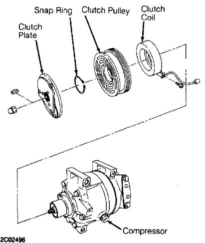
Fig. 3: Exploded View Of Compressor Clutch (Calsonic V5) Courtesy of Nissan Motor Co., U.S.A.
