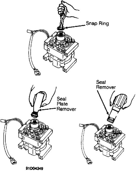
Fig. 16: Removing Rotary Vane Compressor Shaft Seal Courtesy of Mazda Motors Corp.
